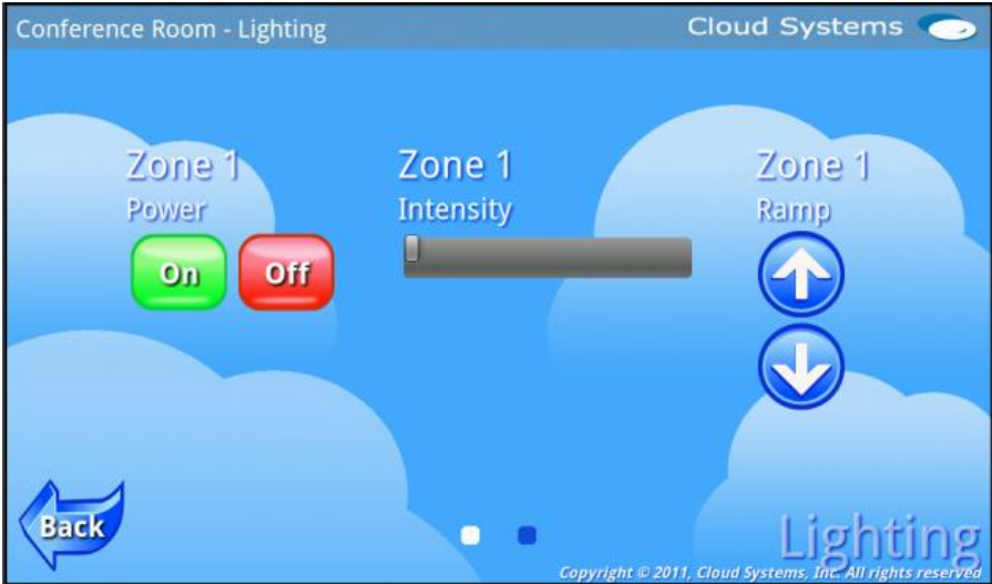
Figure 11 - Lighting Control Widget Screen
